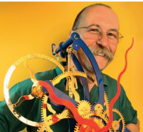
Tourbillon horizontal desk clock Chronometer escapement, half-hourly striking work Power reserve: one week
